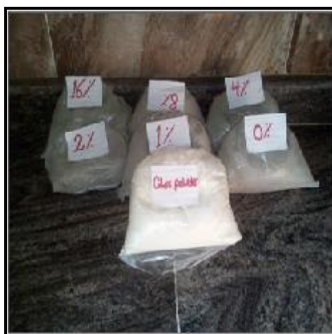
Figure 2. Libda cement factory blended samples with blank sample and glass powder
