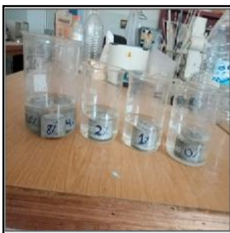
Figure 4. Immersing of cement samples in \text{Na}_2\text{SO}_4 solution
