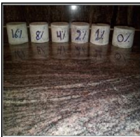
Figure 3. Cement samples after pouring
