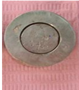
Figure 2. Copper mould 12 mm diameter cavity and 1.5 mm thickness
