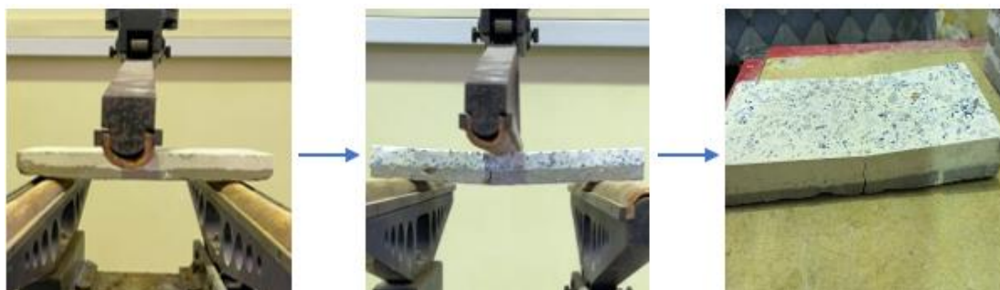
Figure 5. A fracture pattern in the samples due to flexural load
